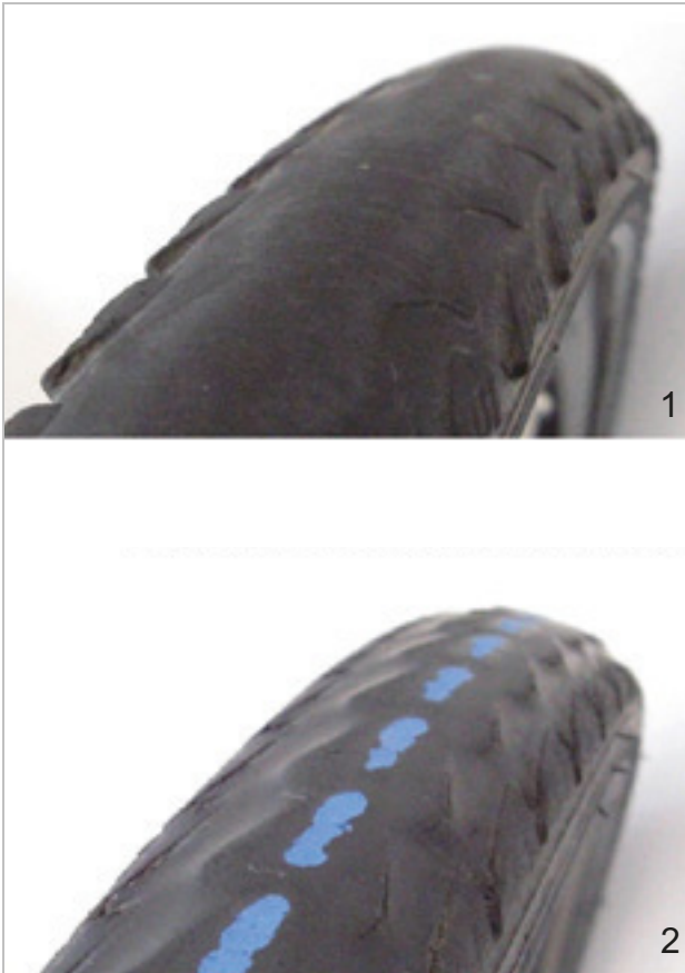
Figure 150: Tyres without a tread which can be replaced (1) and tyres with puncture protection showing through (2) must be replaced
