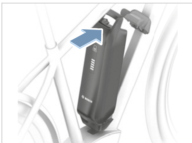
Figure 130: Closing the PowerPack battery upwards
