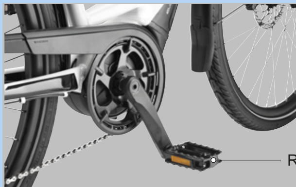
Figure 65: R-pedal in the right-hand crank arm
