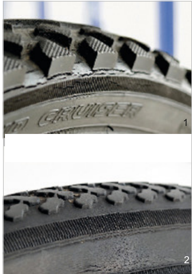
Figure 151: Examples of fatigue cracks (1) and ageing cracks (2)
