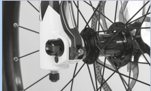
Figure 180: Adjusting the quick release clamping force
