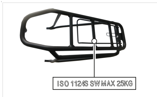
Figure 125: The maximum load bearing (1) capacity is indicated on the pannier rack
