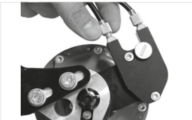
Figure 177: The tension adjuster on ROHLOFF hub versions with external switch control is located on the cable box positioned on the left-hand side
