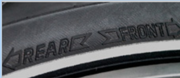
Figure 62: Rotation direction arrow on MTB tyres
