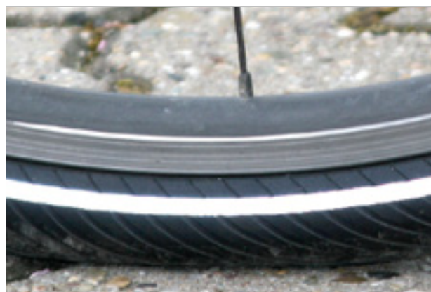
Figure 89: Correct tyre pressure. The tyre is barely deformed under the load of the body weight.
