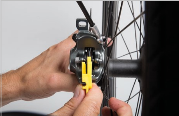
Figure 152: Checking the brake lining when fitted with the help of the transport safety wear gauge
