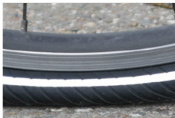
Figure 90: Much too little tyre pressure
