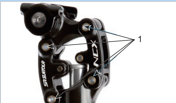
Figure 182: SR SUNTOUR suspension seat post lubrication points
