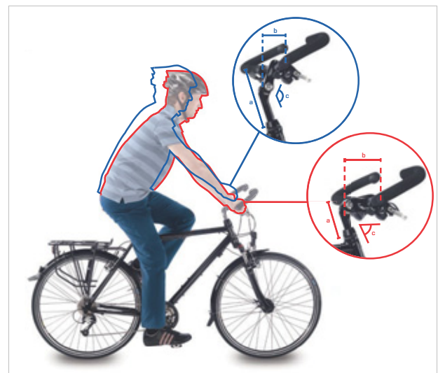
Figure 87: City bike (blue) and trekking bike position (red) by changing the angle
