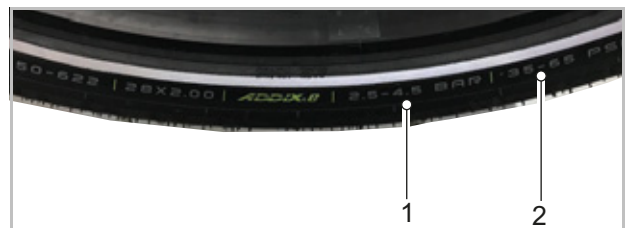
Figure 149: Tyre pressure specification in bar (1) and psi (2)
