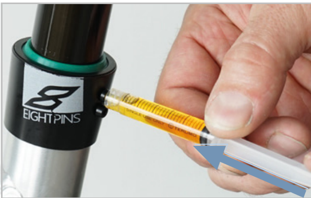
Figure 148: Lubricating the Eightpins seat post
