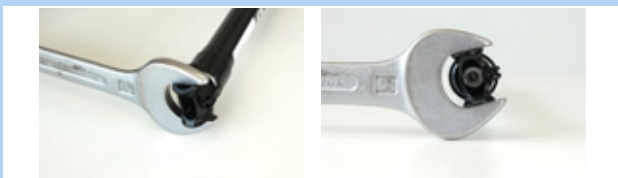
Figur 121: Sikring mod at dreje
